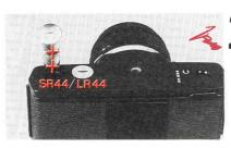
Wipe battery surfaces clean. Make sure that + signs are facing upwards.
