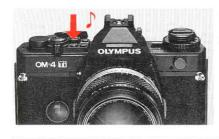
Press the spot button to take meter reading. You will hear an electronic sound and the word "SPOT" will appear in the viewfinder. The metered value is displayed by the "
