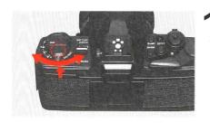
Lift up the outer collar and rotate until the ISO speed appears in the window.
