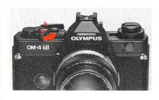
Operate the lever to set up the memory mode. The letters "MEMO" will appear in the viewfinder and the memory signal will blink twice.
